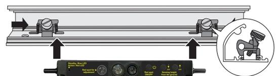
Loosen the screws before connect the mounting brackets to the housing. Put the sensors into the aluminum housing and tighten the two mounting brackets to the sensor.
