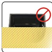
Sensors should not be placed behind the shield.
