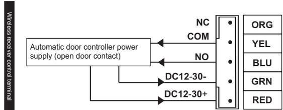
Receiver and automatic door controller wiring diagram
