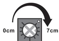
The clockwise direction the induction distance becomes farther, the counterclockwise direction the induction distance becomes closer, and the maximum induction distance is 7cm.
