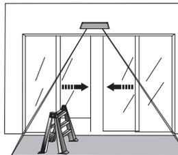
After 15s or 30min(optional), when the sensor is in the sensing area with only stationary object and no other objects or human body entering, the system will learn the objects as the background automatically, then to adapt to the new background, won't transmit door open signal, door will be closed. (As picture showed)
