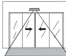
When remove this object away again, and restore to the original scene, the system will intelligently recognize the original scene and transmit a door opening signal for 2 seconds, then return to normal standby state.
