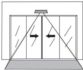
When debugging, in order to avoid the wrong foreground information in the system, before the self-learning process, Please make sure the door in the closing state; In the whole self-learning process, all irrelevant background objects must be removed from the detection range, such as workers, ladders, toolboxes, etc.
