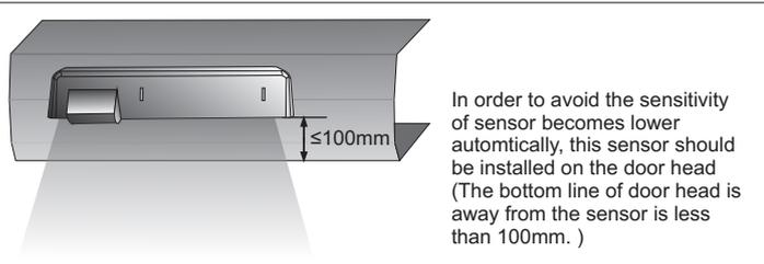
In order to avoid the sensitivity of sensor becomes lower automatically, this sensor should be installed on the door head (The bottom line of door head is away from the sensor is less than 100mm.)
