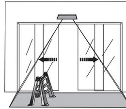
When put a extra stationary object in the detection area, the sensor will transmit a door open signal in time. (As picture showed)
