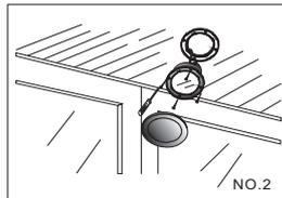
Put sensor into installation hole after wiring connection and fix position by screws.
