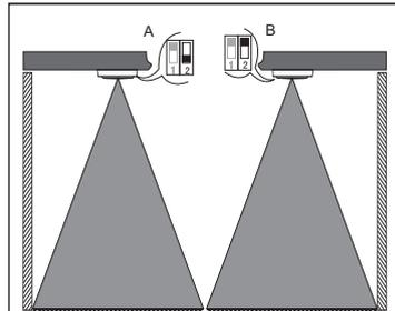
When two sensors installed in very close position, Sensors should be set to different rates. One sensor with A, Antother one with B. (as picture)
