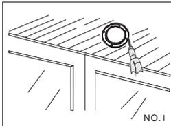
Trepanning according to the screw position of bottom cap. Hole size: more than 53mm (deep)
