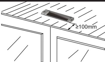
When top suction installation, in order to avoid self-induction, the installation distance between the automatic door and the safety curtain should be more than 100mm.
