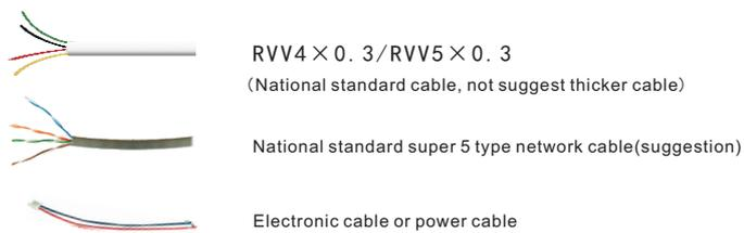
(Remark: When wiring, they can not be with strong the same line pipe, at least 50 centimeters away)
