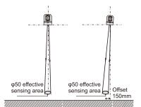
Diagram of side scan area adjustment
