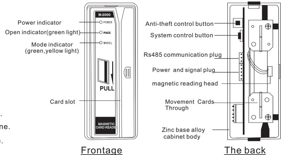
Designed with anti-theft control button(as the picture shown). The button will bounced and the control system will issue a buzz ASAP the magnetic card access controller left the installation wall
