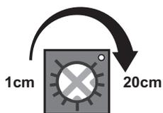
Adjust clockwise, sensing distance become far; Adjust counterclockwise, sensing distance become near. The maximum sensing distance is 20cm.
